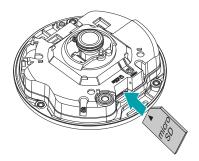
· Push the SD memory card until it disengages from the slot, and then pull it out.
