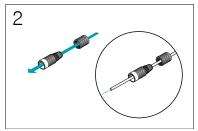
Insert the network cable into the waterproof cap, 2 rubber bushing, and waterproof cap body in order.
