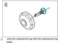
Not pulling the cable back may cause water to seep in and damage the product.
